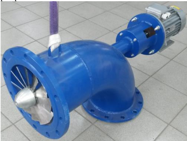
Fig. 9 (a) The hydraulic unit with propeller axial-type impeller
